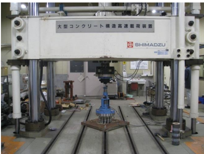
Figure 2 Overview of Constant Deformation Rate Test Equipment [3].
