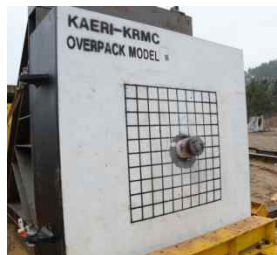
(a) KORAD21C over-pack with liner and reinforced bar
