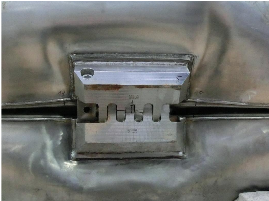
Figure 10: Closure device after the drop test sequence onto the side of the PSP with final impact of the bar onto the closure device
