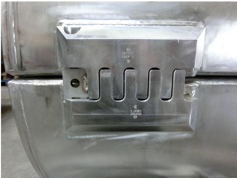
Figure 9: Prototype closure device before the drop tests
