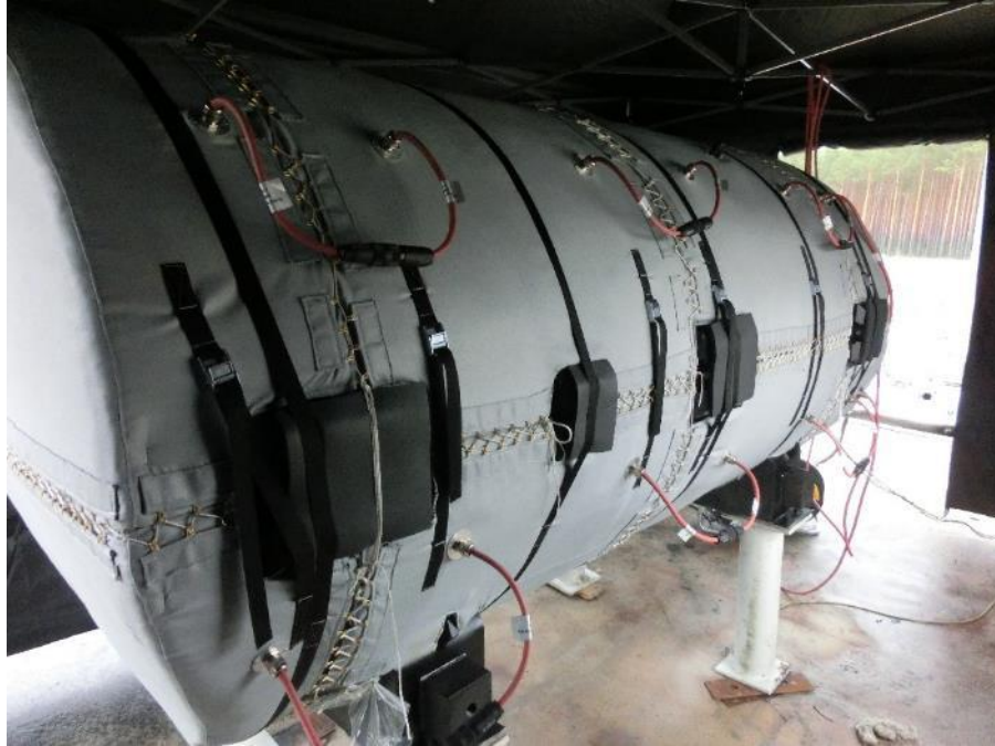
Figure 5: DN30 prototype in heating jacket
