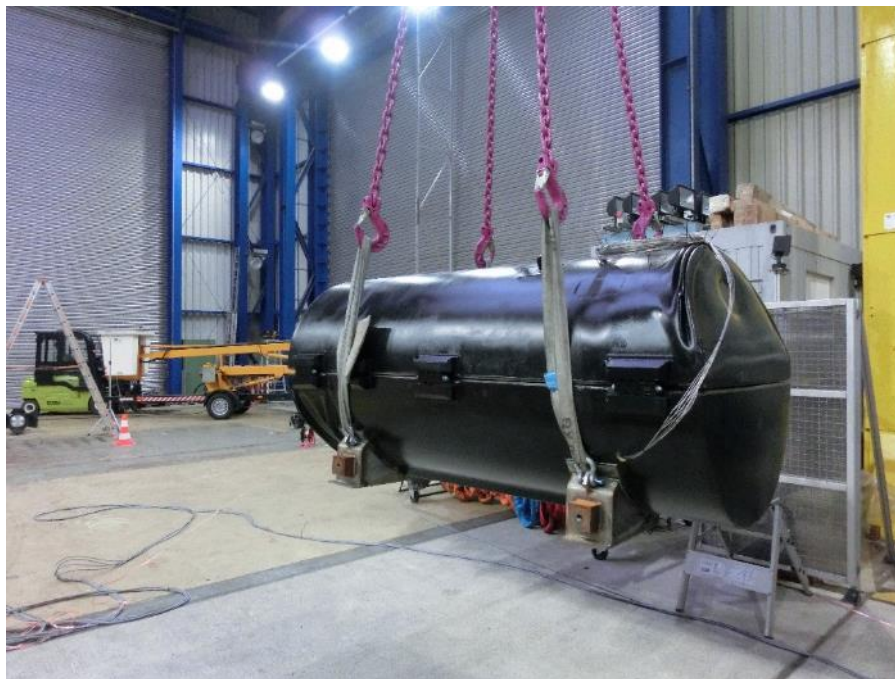
Figure 4: DN30 prototype coated for the thermal test
