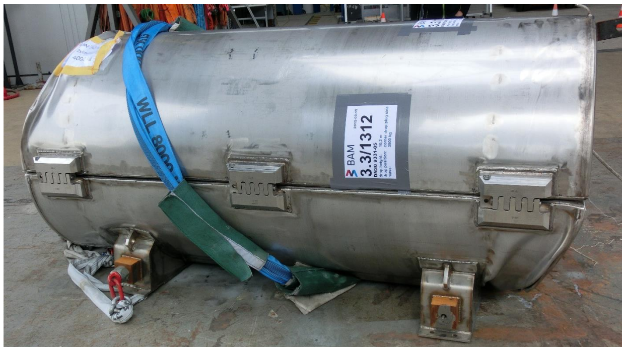
Figure 3: DN30 prototype used for the thermal test
