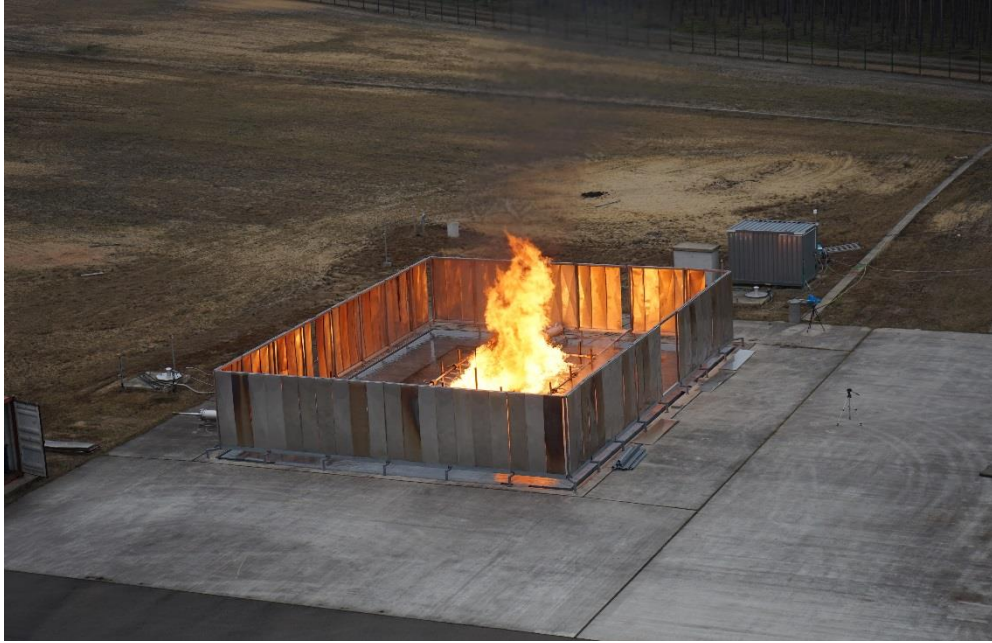
Figure 6: Picture of the fire test showing the full flame engulfment of the DN30 prototype
