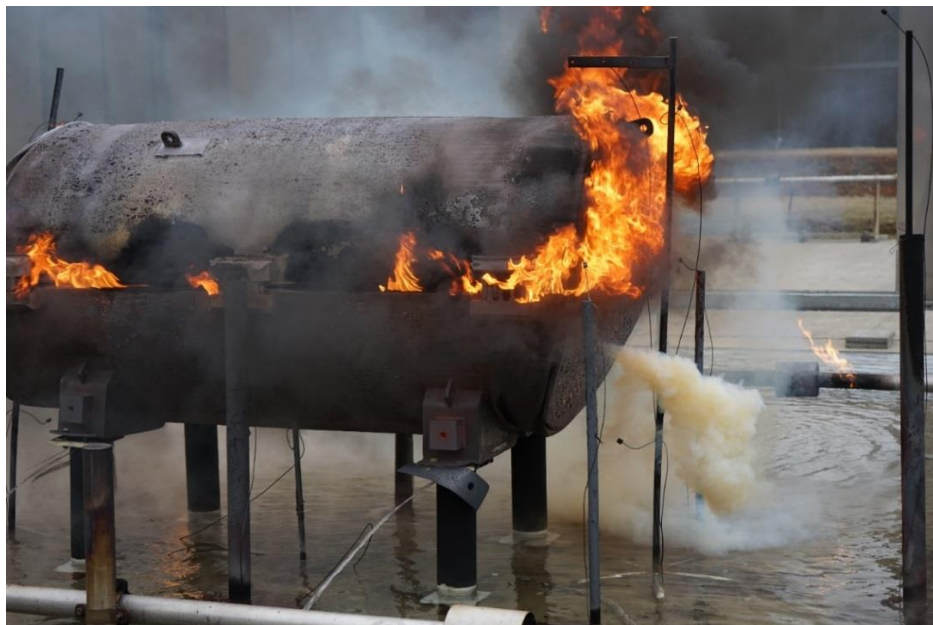
Figure 7: Gases escaping from the DN30 prototype during the cooling phase
