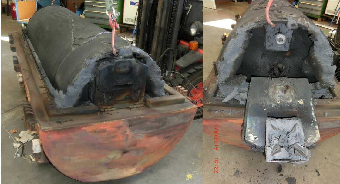
Figure 12: Expanded intumescent material inside the DN30 PSP after the oven test
