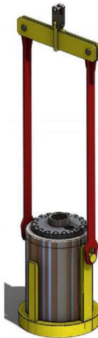
Figure 3 – Principle of lifting beam and supporting chair
