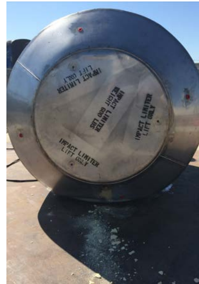
Figure 4 – CTU Condition after D3 Free Drop Test
