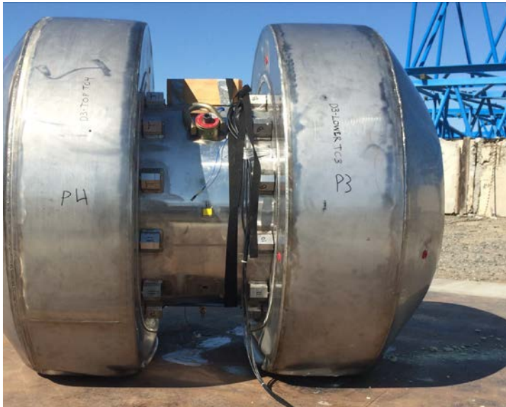
Figure 4 – CTU Condition after D3 Free Drop Test
