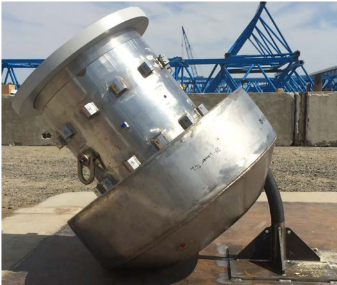
Figure 3 – CTU Condition after P3 Puncture Drop Test
