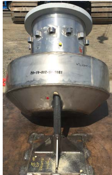
Figure 3 – CTU Condition after P3 Puncture Drop Test
