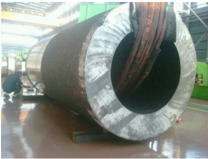
Fig.6 Forged cask body
