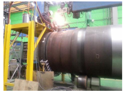
Fig.8 Narrow gap welding
