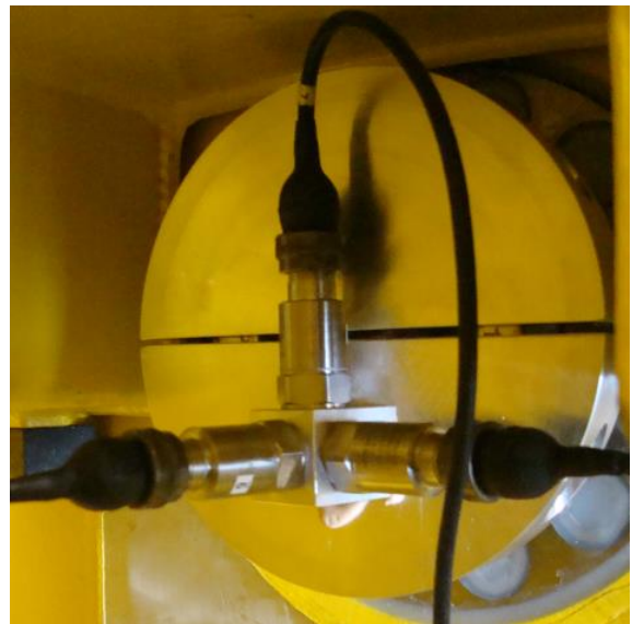
Figure 5: CASTOR® package (left) and accelerometers on the cask (right)
