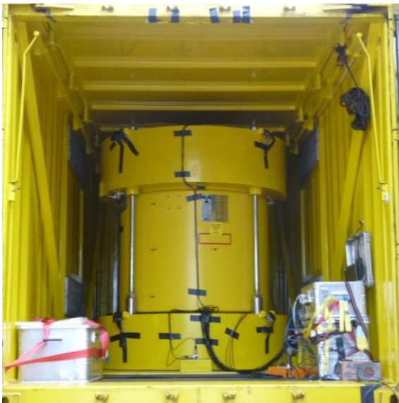
Figure 5: CASTOR® package (left) and accelerometers on the cask (right)
