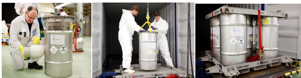
Figure 8: 9975 packages ready for transport
