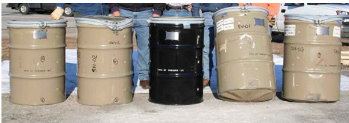
Figure 6 Prototype Packages following HAC Structural Tests
