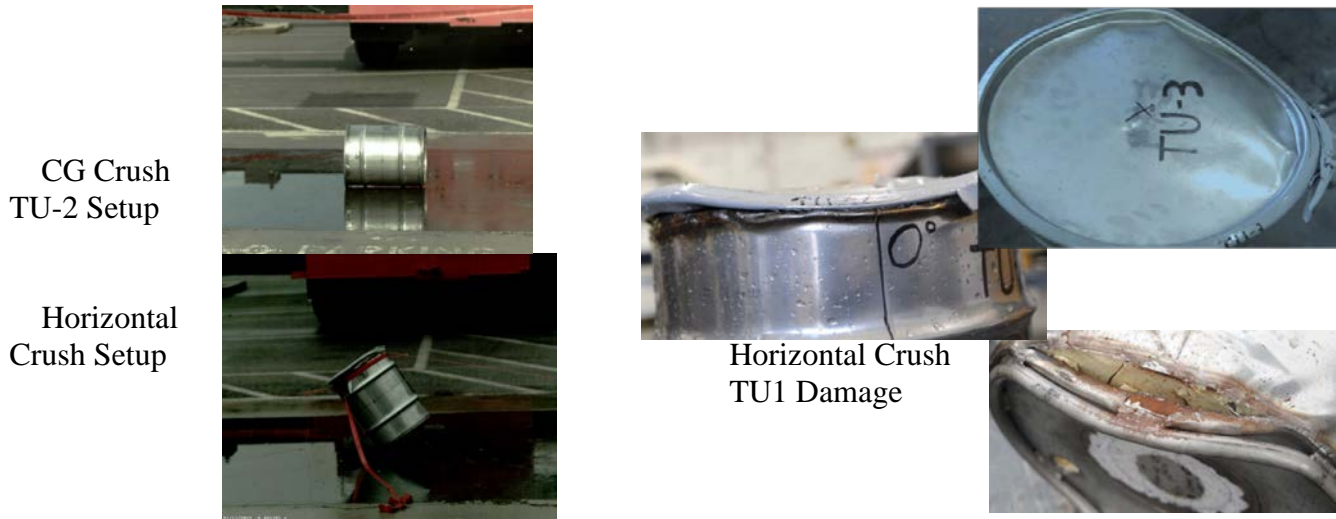
Figure 5 Hypothetical Accident Condition 30-Foot Drop and 30-Foot (1,100 lb. Plate) Crush
