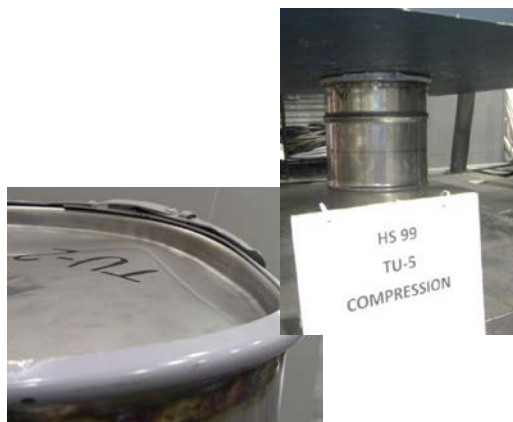
Figure 4 NCT Testing (Water Spray, Compression) - Damage from 4-Ft drop and Puncture bar
