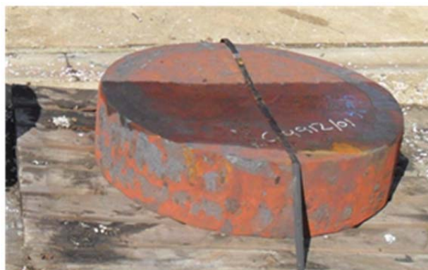
Figure 4 - Open die forged steel disc before machining of lid detail
