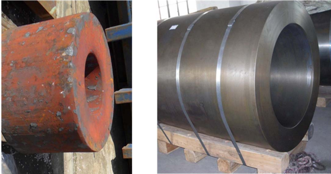
Figure 5 - Open die forged tube before and after final machining
