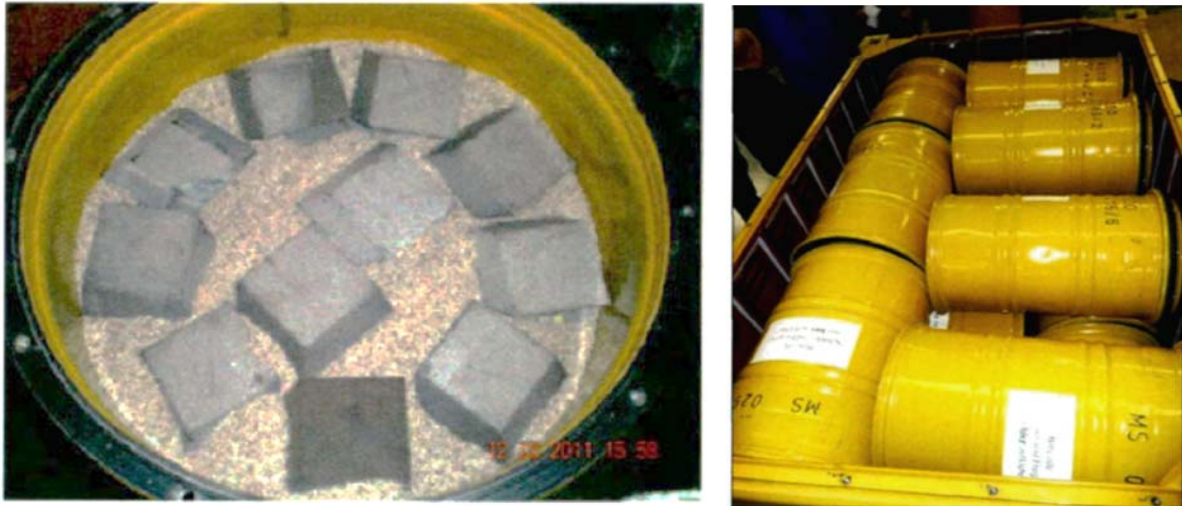
Figure 1: Content of a typical drum during loading showing the lead blocks encapsulated in sand, and loading arrangement of drums inside the container.
