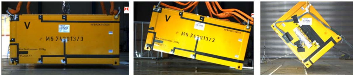
Figure 2: Impact orientations for drop tests.
