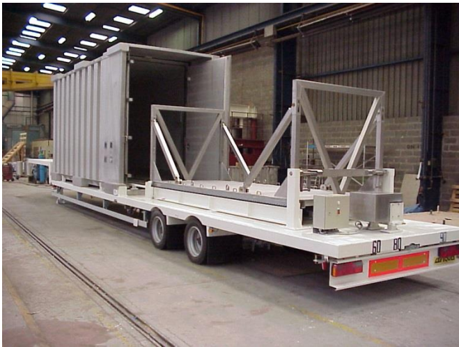
Automated Loading/Unloading System Integrated with Container/Trailer
