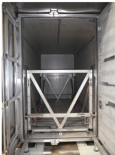
Securement of the Automated Loading System (and Payload)
