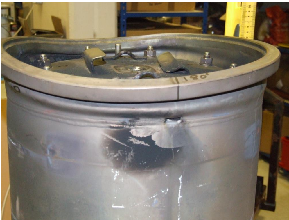
Figure 14. Damage to Top Rim and Skirt of Keg after Testing
