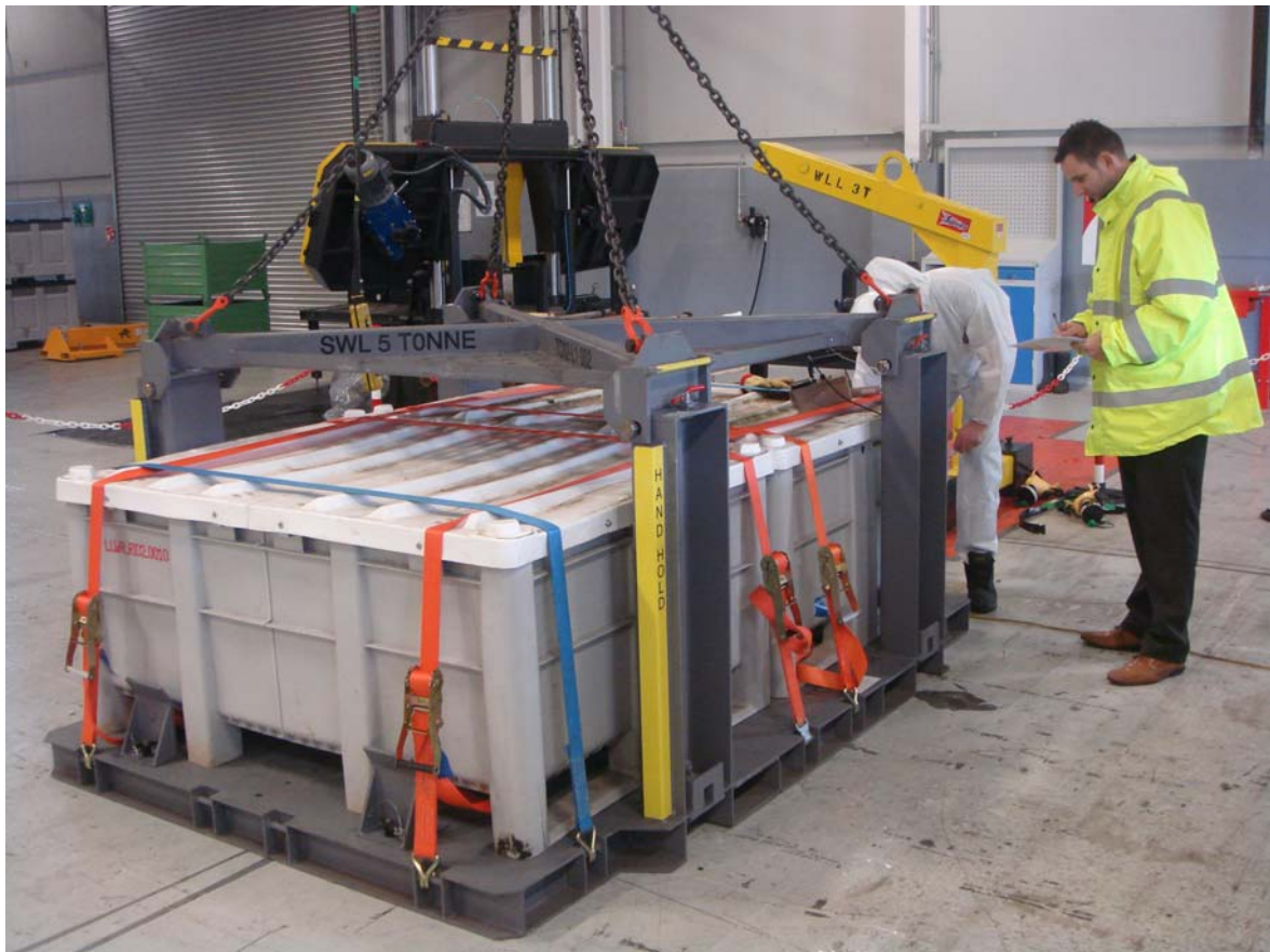
Figure 4: Type S1 stillage with secondary inner waste box loaded and lifting frame attached
