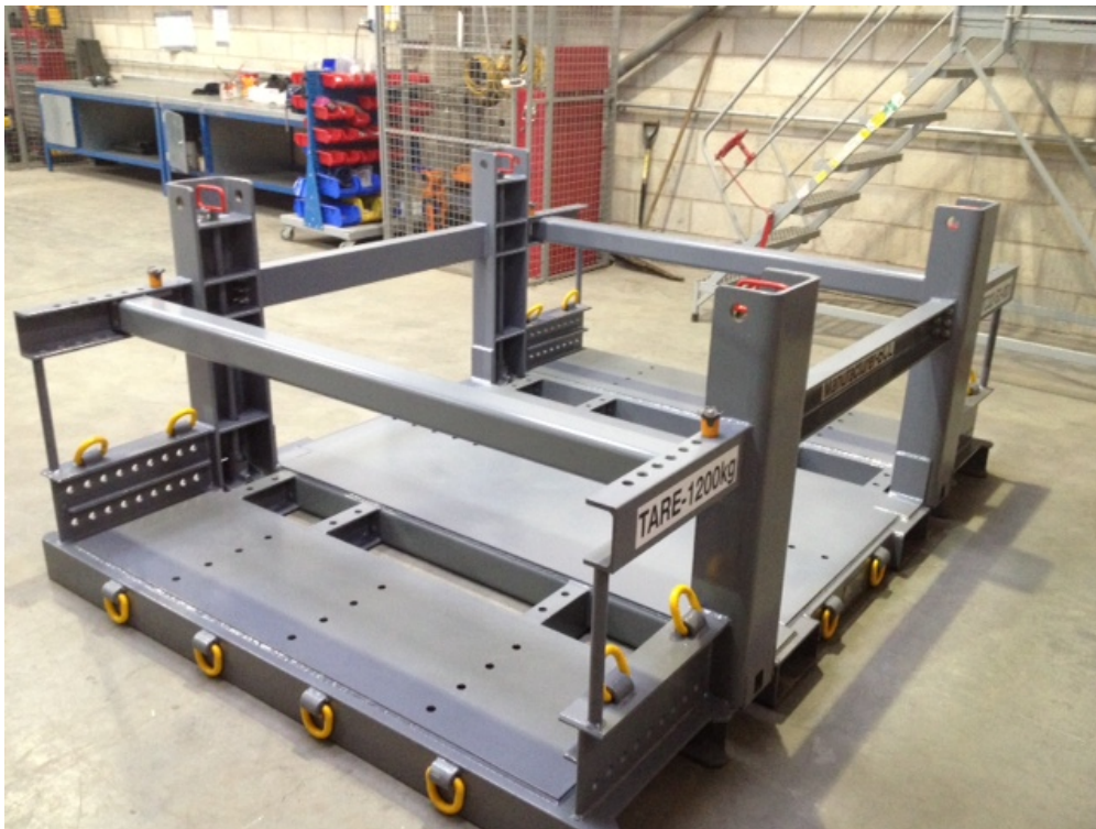
Figure 6: Type S3 stillage configured for drum payload
