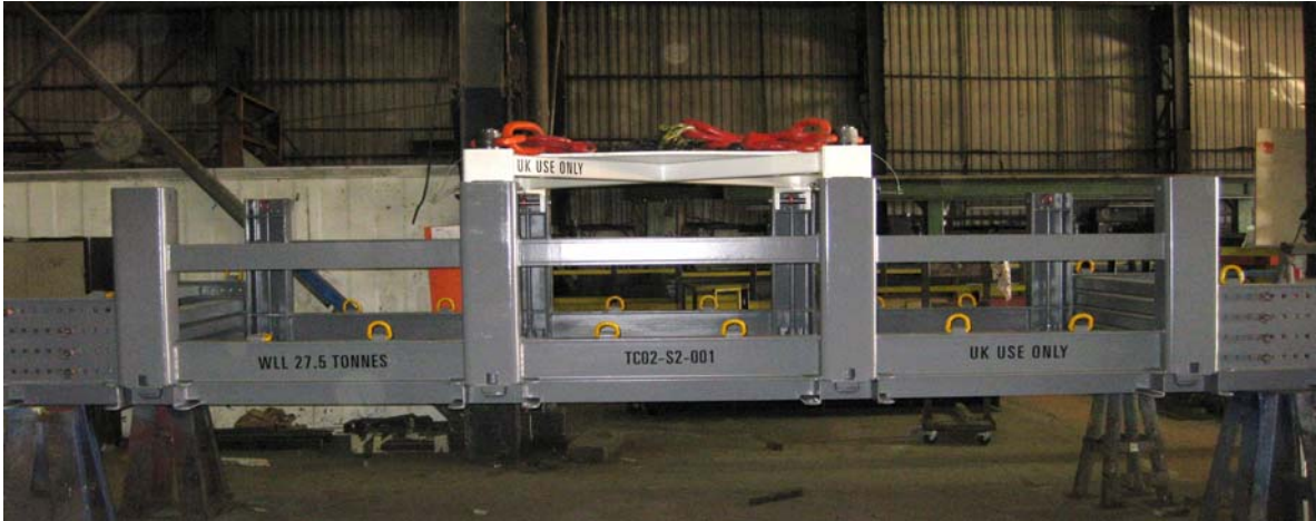
Figure 5: Type S2 stillage with lifting frame engaged
