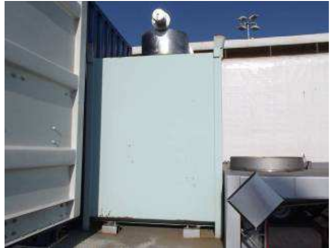
Transport Container for Recovered UF 4
