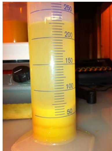
Figure 3: SDU settling with iron sediment layer
