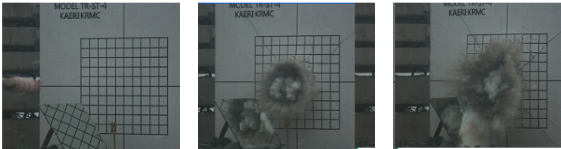
Fig. 12 Moment of impact for Type 2 segment model
