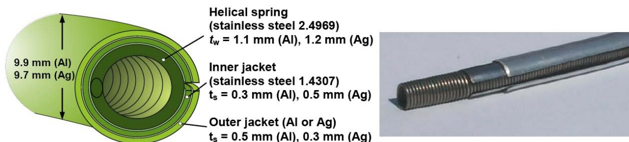
Fig.1 Helicoflex ® gasket type applied in test series, typical for applications in dry storage metal casks [3, 4]
