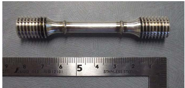
Fig.4 Dimension of the test specimen for tensile and creep tests for pure silver material
