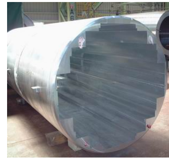
Fig. 3.1.6 Machining Prior to Channel Parts Installation
