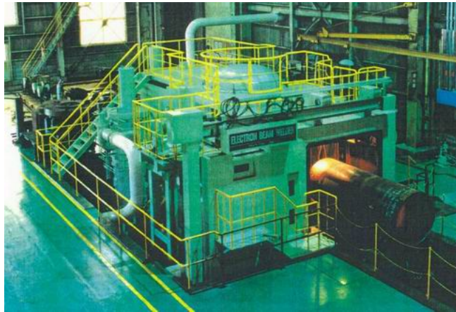
Fig. 3.1.4 Electron Beam Welding System
