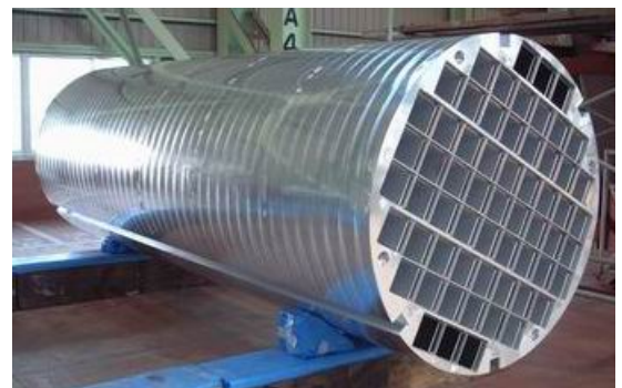
Fig. 3.1.8 Dry Storage Cask Basket
