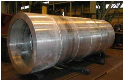
Fig. 3.1.5 Aluminum Forged Rings to Shell
