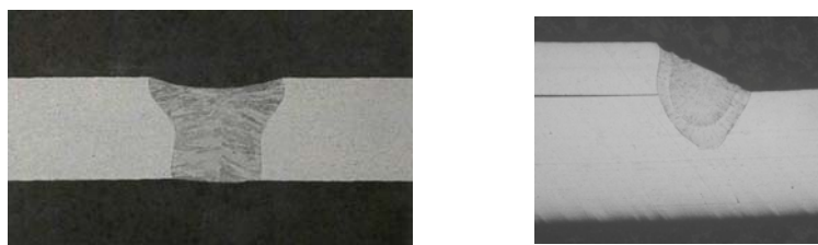
Fig. 3.2.2 LBWs on MPC Square Tube and Cradding
