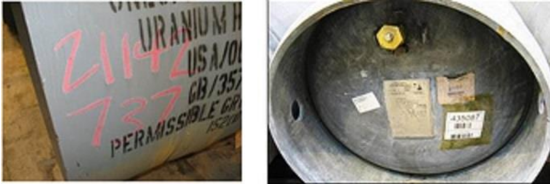
Figure 3. Examples of additional markings and labels applied by operators to improve ability to identify cylinders.
