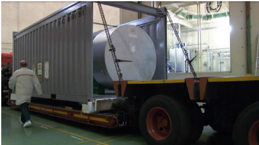
Figure 7. Shipment of the NAC – LWT cask loaded onto the “omega” road trailer
