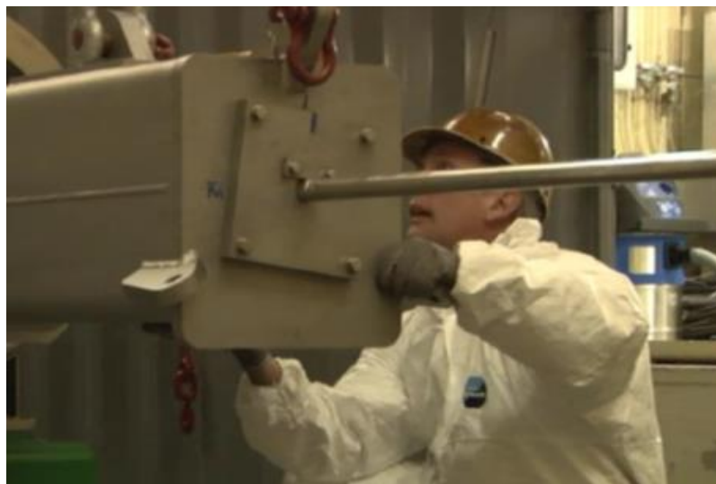
Fig 1. Coupling of the Shielding Transfer Device to the NAC – LWT package
