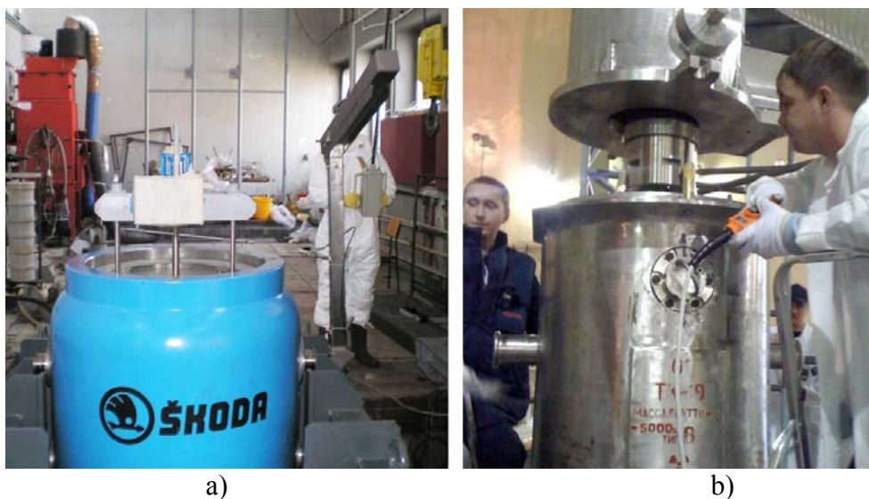
Fig. 9. Loading SKODA VPVR/M cask over the basin (a)
