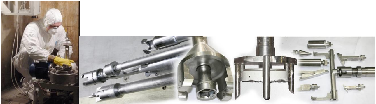
Fig. 8. Equipment and tools for SNF repackaging
