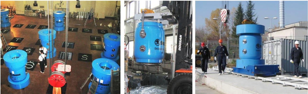
Fig. 10. Arrangement of casks in the reactor hall. A forklift and a transport trolley for the casks
