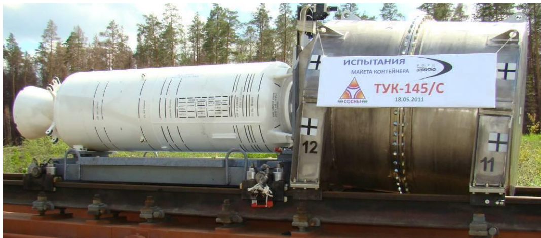
Fig. 5. Mockup TUK-145/C (1:2.5 scale) on the rocket sled
