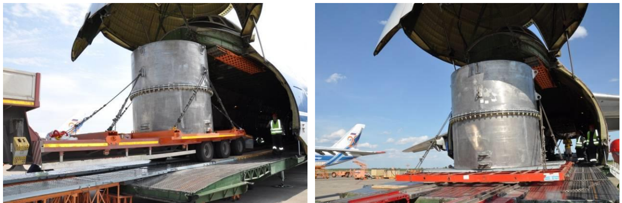
Fig. 9. Loading of the TUK-145/C package into the AN-124-100 aircraft
