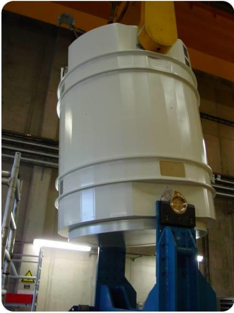
Figure 1 : The TN ® 24 SH dual purpose cask handling operation
