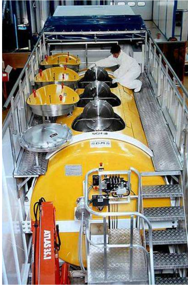
Figure 2: LR56 tank for moderately radioactive liquids
