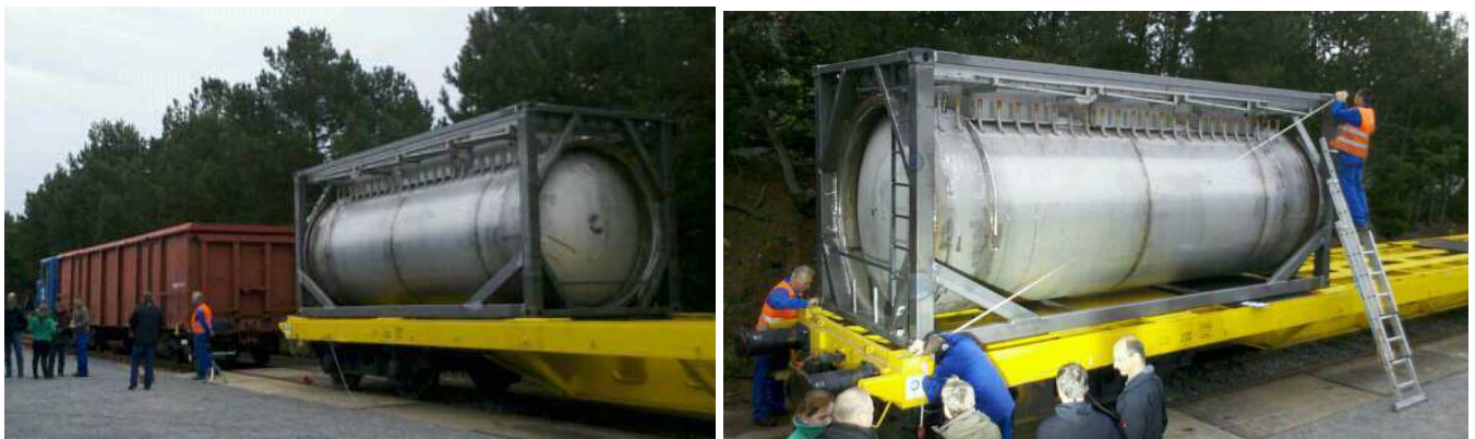
Figure 12: Dynamic test campaign of LR154 tank
