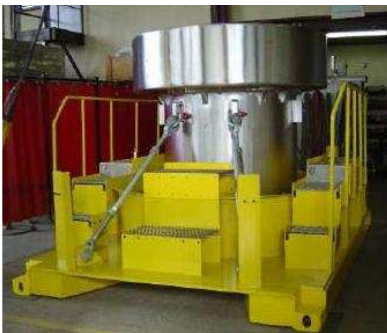
Figure 4: SORG transport package for organic liquids
