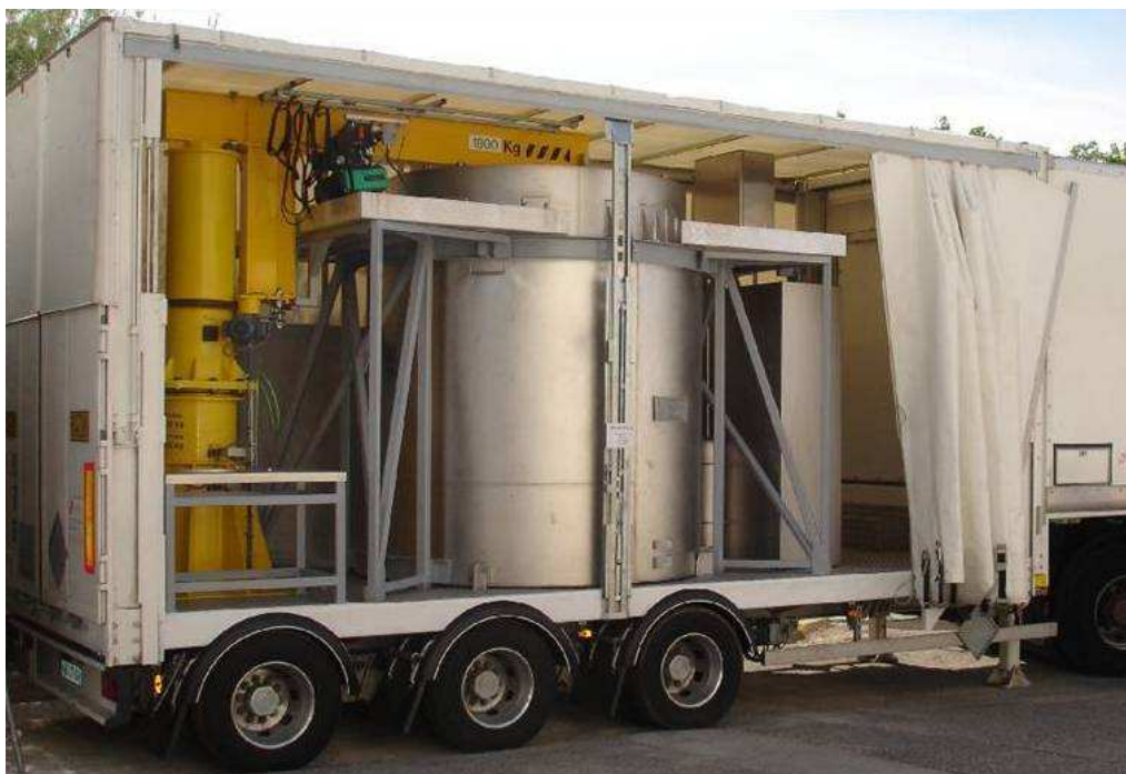
Figure 3: LR144 transport package for highly radioactive liquids
