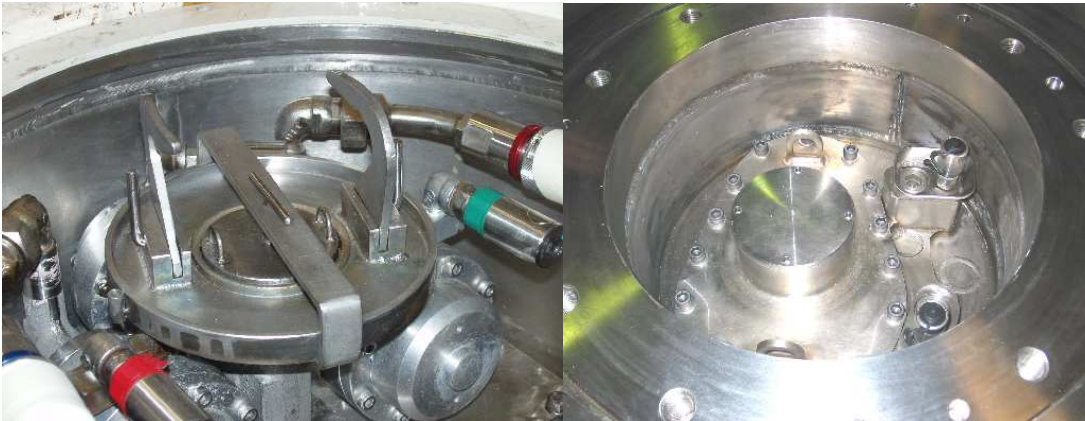
Figure 9: Tank access wells of LR44 (left) and of LR144 (right)
