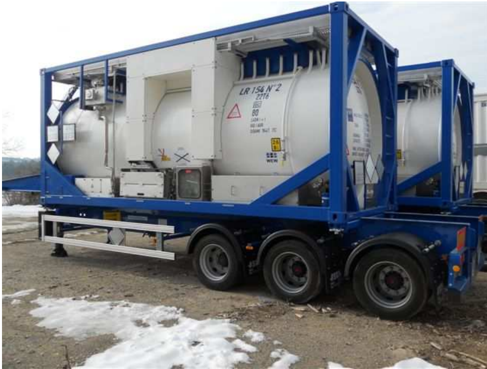
Figure 1: LR154 IP2 tank for LSA II liquids
