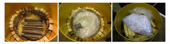
The drum was progressively filled to the 70% level with wood blocks, wood shavings, steel bars and absorbent mats and a 65kg bag of lead shot. A bag of shredded paper and further wood shavings filled the drum with test dust added prior to securing the lid.
