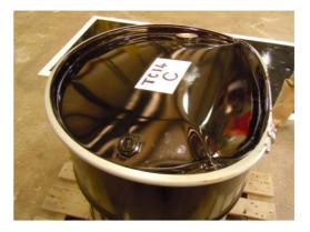
No test dust was found on the outside of the drum or on test plate following the drop test. Lid distortion was concentrated towards point of impact. Small creases occurred in the lid as a result of the impact but none which compromised the seal to the drum curl.
