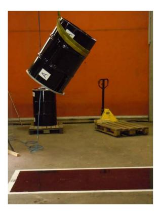
In all cases the 1.2m drop test was performed by suspending the package from the drop test hook and allowing it to drop onto an unyielding steel test plate. The orientation was such that the centre of gravity was directly above the point of impact which had been set up to be the nut and bolt on the closure ring (Specimen A shown).
