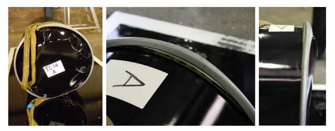
Severe distortion to the lid and closure ring resulted in the lower part of the closure ring and lid detaching from the drum body opposite the impact point indicating a gross failure.
