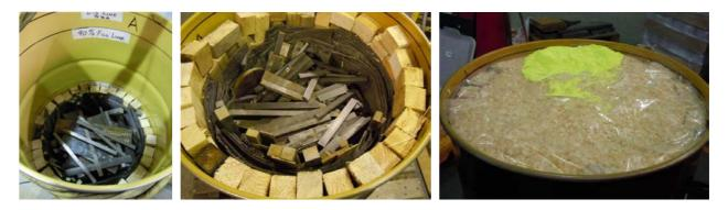
A layer of test dust was placed in the base of the drum which was filled progressively with wood blocks, wood shavings, steel bars and oil soaks. The load was topped off with a steel plate with wood shavings on top and more test dust added prior to securing the lid.
