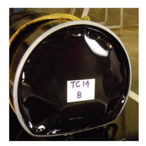
The tests of specimens B and C were successful and this is due to the fact that the drum body was able to deform due to the payload being essentially granular or ovoid, (and therefore able to yield) reasonably homogeneous and of uniform density.
