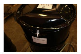
Specimen B met the test requirements with no loss of contents.
