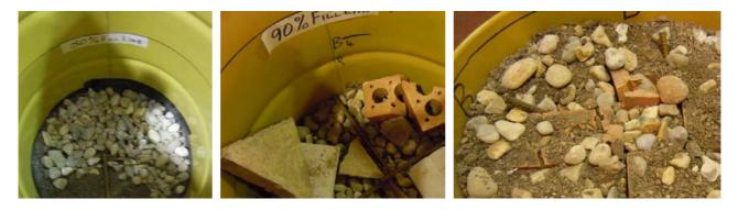
A layer of test dust was placed in the base of the drum which was filled progressively with soil, rebar, pebbles and rubble with rebar tapped into the top soil/rubble layer simulating a sharp penetrative object in the top of the drum. More test dust was added prior to securing the lid
