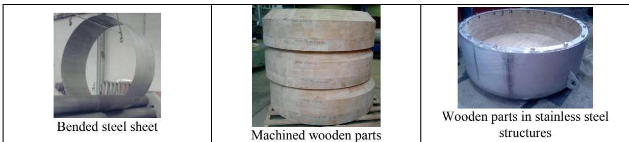
Figure 8. Shock absorber manufacturing steps
