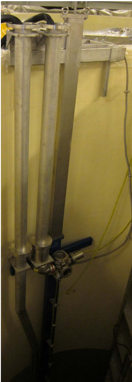
Figure 6 UBE hanging at wall of pool (before filling with water)
