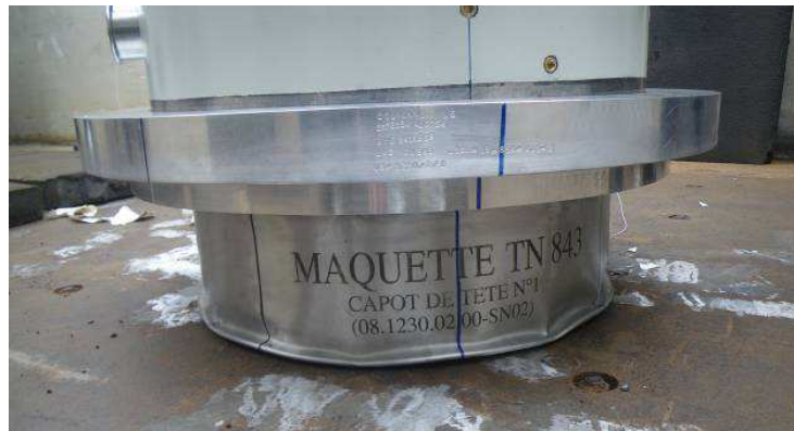
Figure 4: View of the TN®843 3:1 top shock absorber after axial drop
