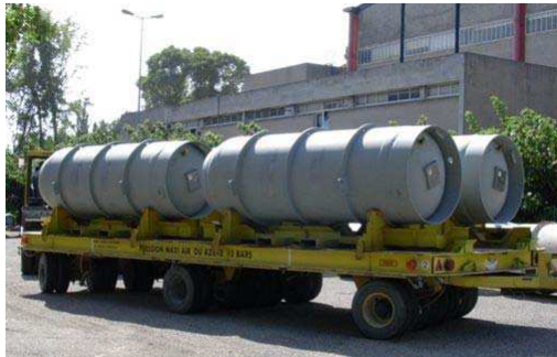
Figure 1. Picture and sketch of UF 6 cylinder 30B (dimensions in cm and inches)
