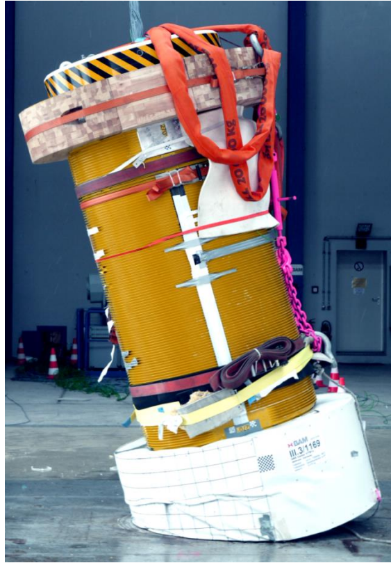
Fig. 4 Test cask on a scale of 1:2: 9-m lid edge drop at a design temperature of the impact limiters of 80 °C
