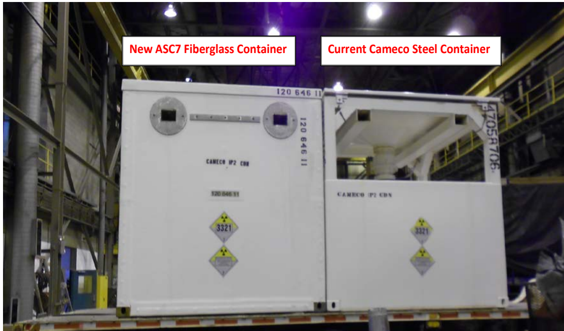
Figure-11. ASC7 Mounted on Trailer Adjacent to a Metal Container for Operational Testing
