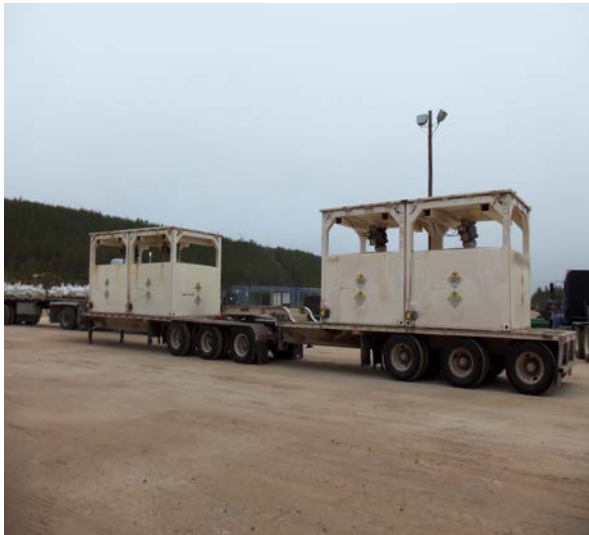
Figure-4. Trailer's Loading Configuration (all metal containers)
