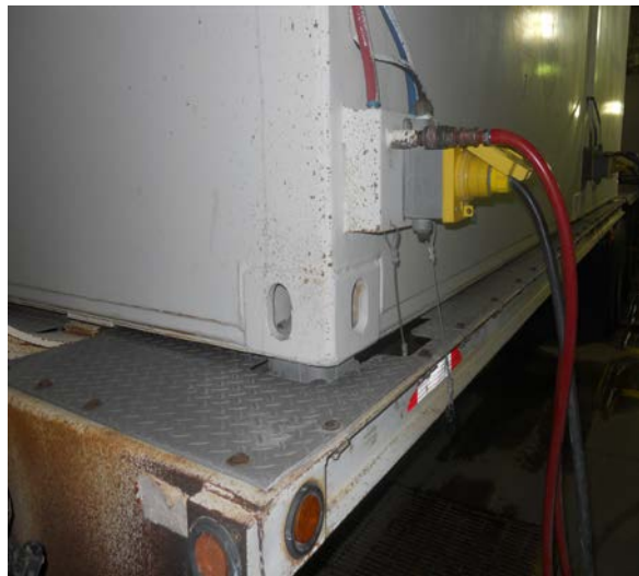
Figure-5. Trailer's Current Mounting Configuration and Quick Connects
