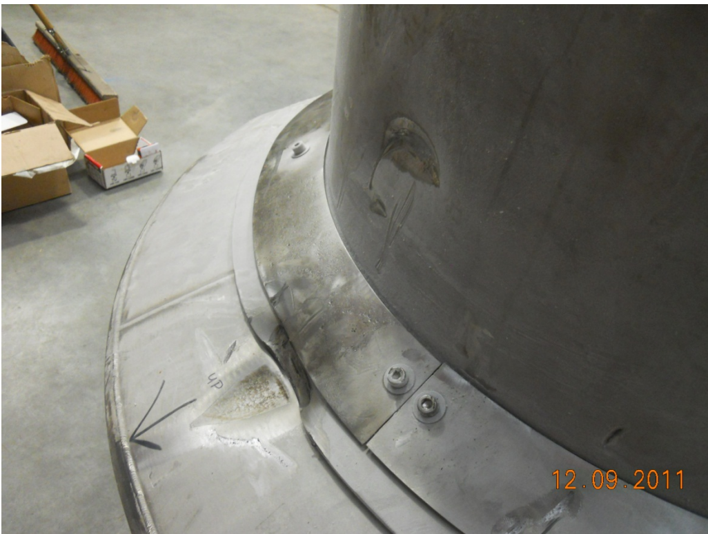
Figure 7. Puncture Damage to Bolt Tube Region
