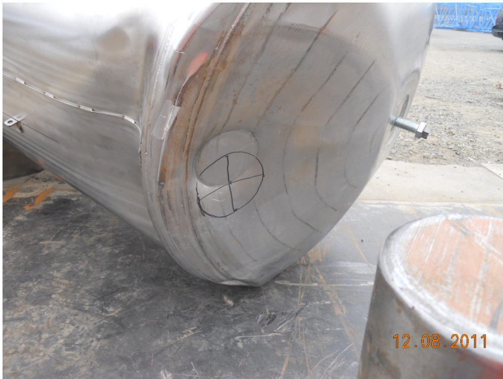
Figure 5. CG-over-Knuckle Free Drop and Puncture Damage
