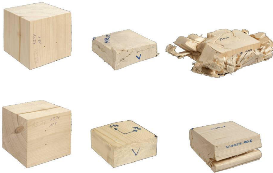
Figure 3. Top: specimens before crush test with load parallel to the fiber (lhs), crushed with lateral constraint (middle), crushed without lateral constraint (rhs). Bottom: crush test with load perpendicular to the fiber, accordingly
