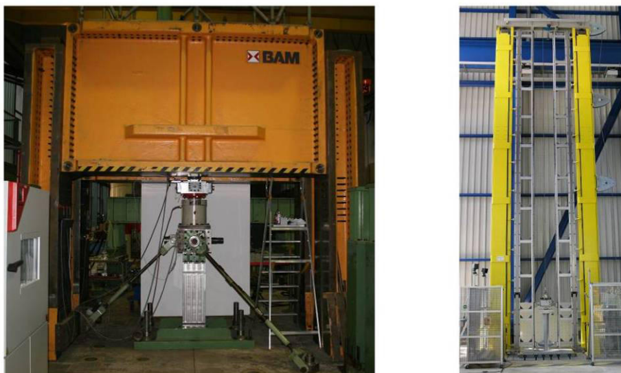
Figure 1. Servo hydraulic impact testing machine for constant loading speed (displacement controlled) of up to 4,500 mm/s and test forces of up to 1,000 kN (lhs). Machine for guided drop tests for variable loading speed (energy controlled); maximum drop height 12 m, maximum drop mass 1,200 kg
