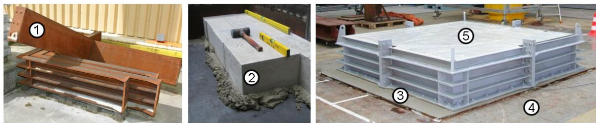
① Brackets ② Damping concrete layer ③ Grout ④ Unyielding target ⑤ Damping concrete footing
