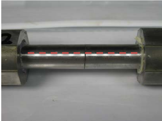
Fig. 18 Test for SSAP11 was conducted on Bose with original setup: load \pm 200 N, moment \pm 20.38 N*m, 5 Hz. Initial displacement \pm 2.5 mm, initial curvature \pm 0.27 /m, initial strain \pm 0.14\% . Specimen fractured near 678K cycles. About 40% drop in flexural rigidity occurred.
