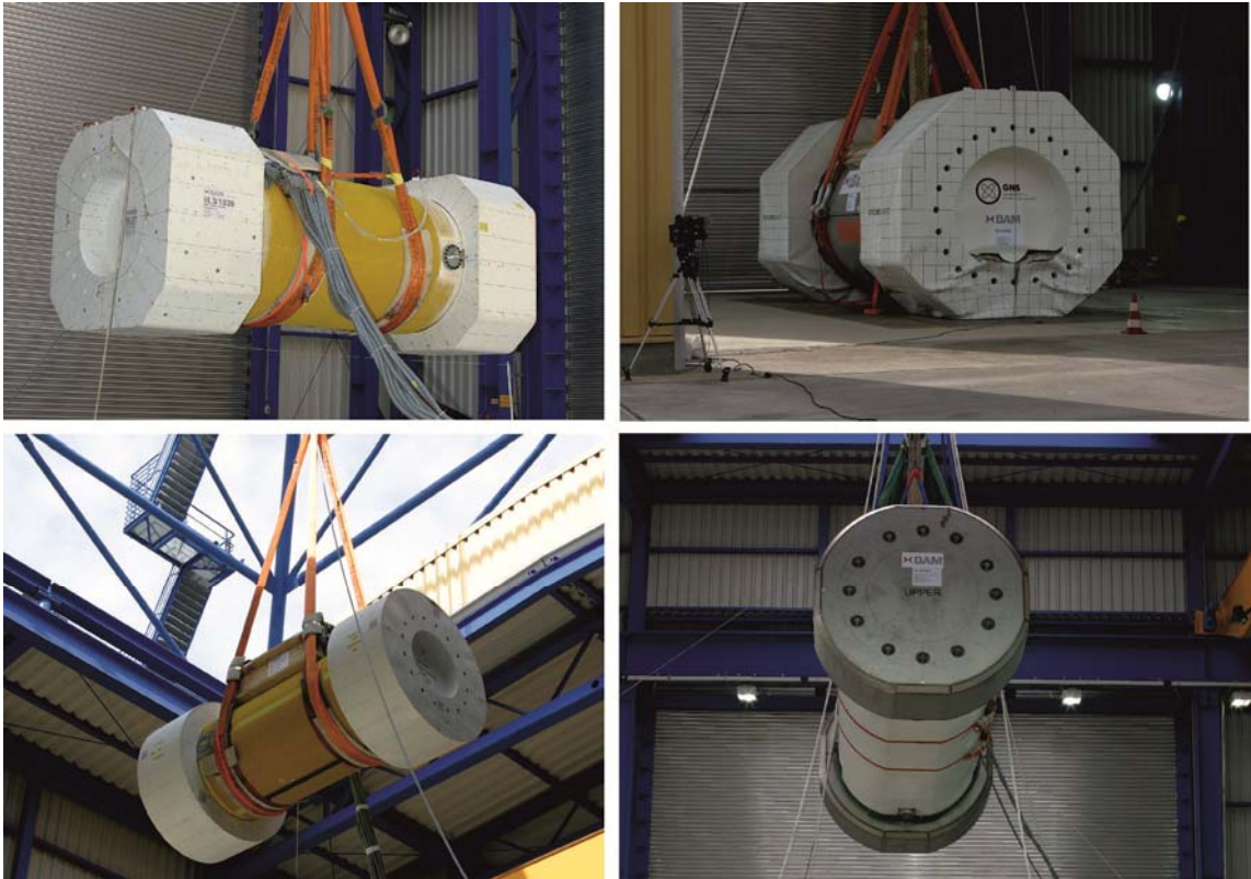
Figure 4: Different impact limiters designs
