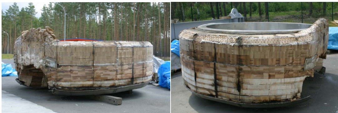
Figure 3: Impact limiter built of thin steel plates filled with wood of different kind and fiber direction [6]
