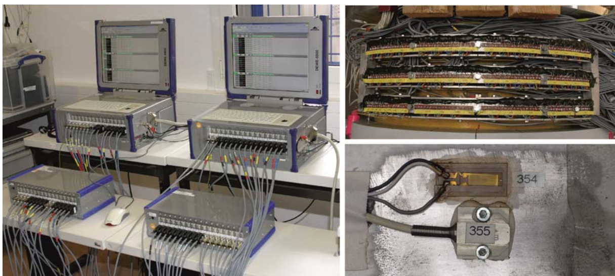
Figure 6: Data acquisition (left), central soldering terminal (top right), accelerometer and strain gauge on an impact limiter (bottom right)
