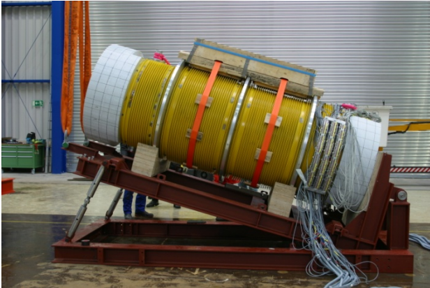
Figure 5: Cask with circumferential impact limiters as well as lid and bottom impact limiters
