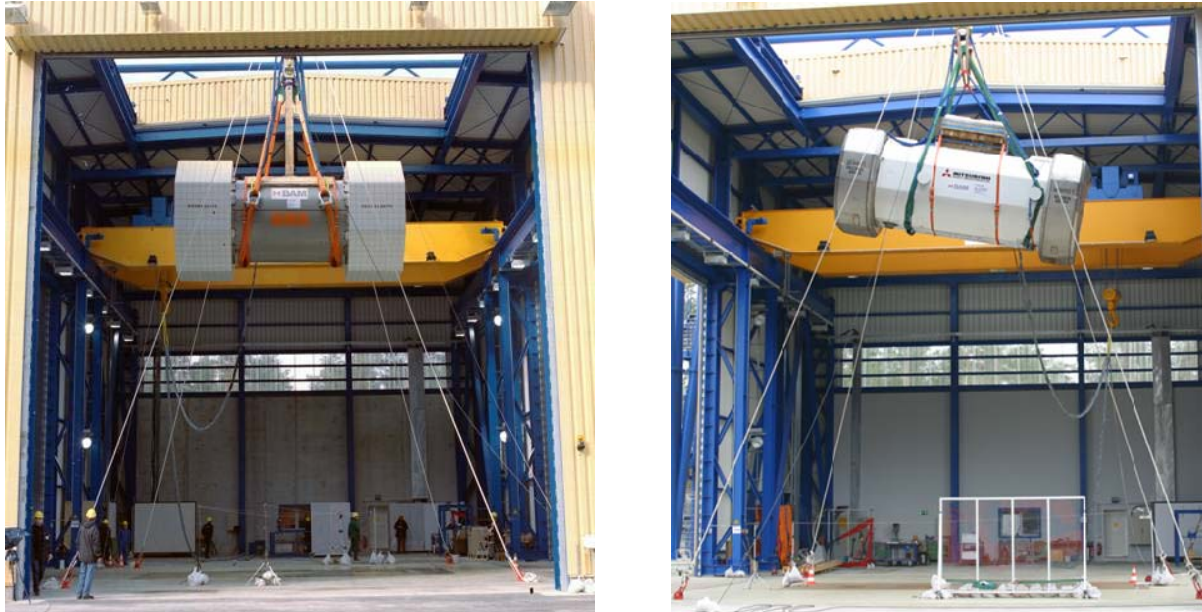
Figure 2: 9 m drop test according to IAEA with typical transport cask configuration (full-scale SNF cask) [6]
