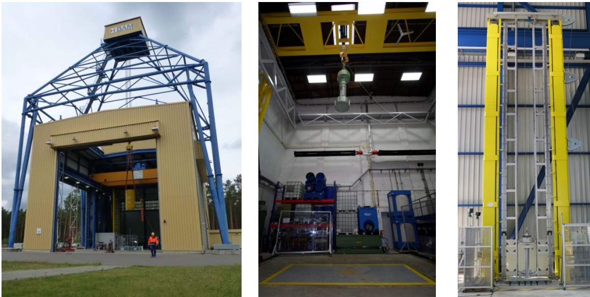
Figure 1: 200 tons drop test facility, indoor drop test facility and drop test machine (from left to right)
