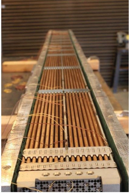
Figure 2. Diagram showing the Zircaloy-4 rods instrumented for the tests (top) and instrumentation on the actual assembly (bottom). The Zircaloy-4 rod shows as “silver” in comparison to the copper rods.
