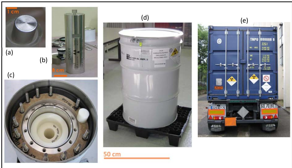
Figure 1: Packaging of a radioactive source (a and b), loading of the capsule into the S300 packaging (c and d), and loading into the ISO 20 ft container (e)
