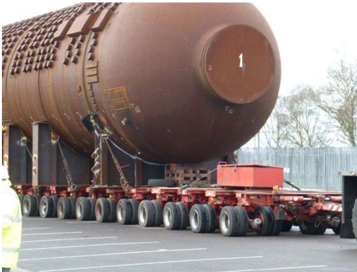
Figure 9 – Road Transport of Decommissioned Boiler
