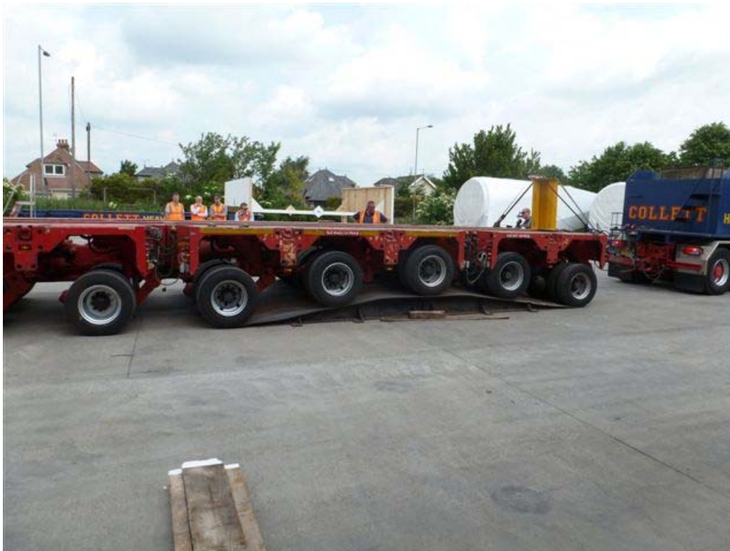
Figure 2 – Trailer Performance Over Humps
