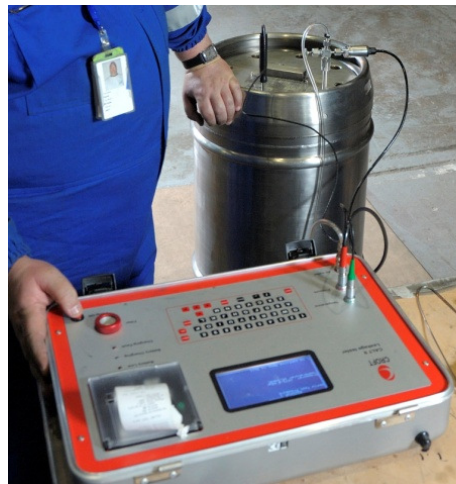
Figure 10: INS 3578 OCV pressure drop test
