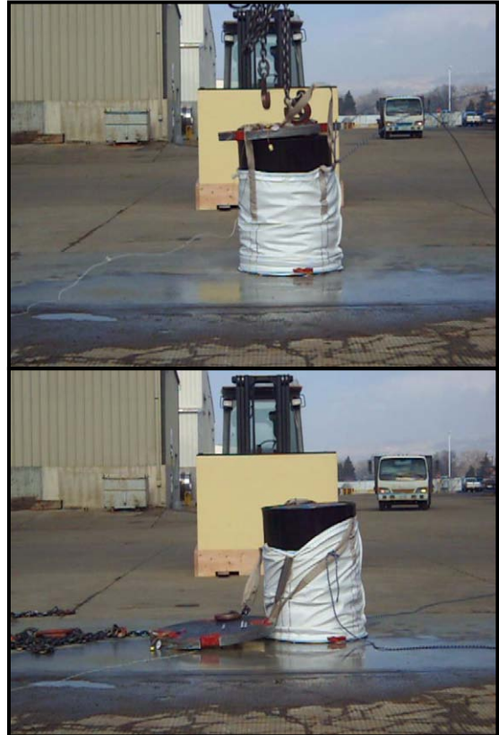
Figure 13. During and Post End Drop
