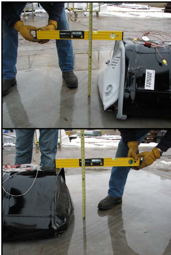
Figure 9. CCO Side Drop Inspection
