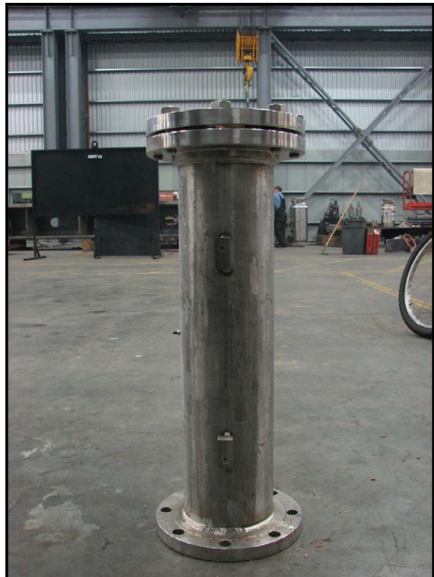
Figure 10. CCC Side Drop Inspection
