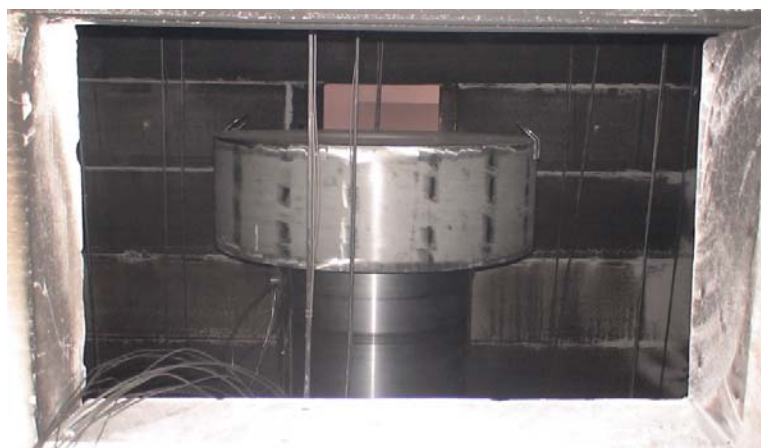
Figure 4. A 1/3 scale model of the metal storage cask was installed in the compartment
