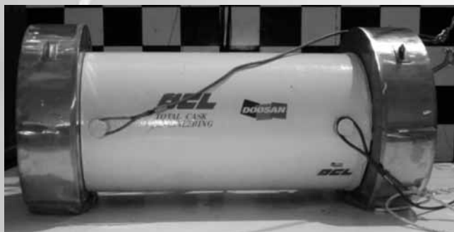
Fig. 2 The cask after the horizontal drop
