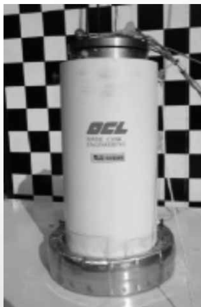
Fig. 1 The cask after the top vertical drop
