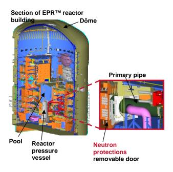
There area three main types of neutron protection implementations around main coolant legs : Hot Leg 1, Cold Leg1 and Cold Leg 3. The neutron shielding will be provided by TN Vyal  $B^{TM}$  blocks embedded in stainless steel boxes.
