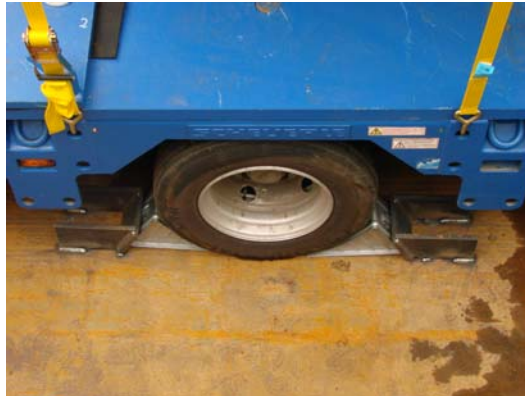
Figure 9. Wheel chock on the barge
