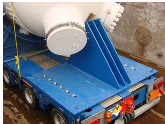
Figure 8. Tie down primary part
