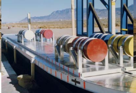
1/5 scale model of lashing apparatus and Air Transport Packaging of a cargo air plane floor
