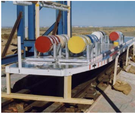
1/5 scale model of lashing apparatus and Air Transport Packaging of a cargo air plane floor
