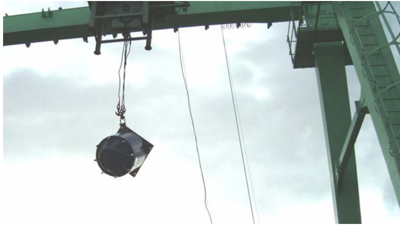
Fig.9 Orientation of the cask under 9m drop
