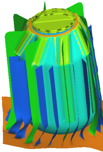
Fig.6 Final deformation under 9m horizontal drop
