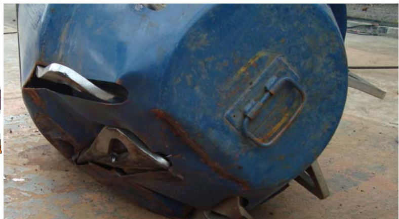
Fig.11 Deformation of the cask after the drop test
