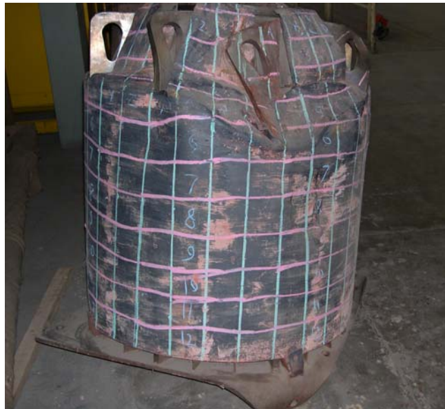
Fig 12 Radiometry carried out on the deformed cask.
